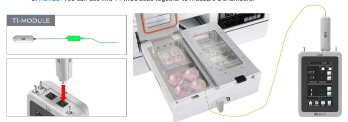
Place the cable of LEO's probe so that the tip of the sensor touches the bottom of the dish.
